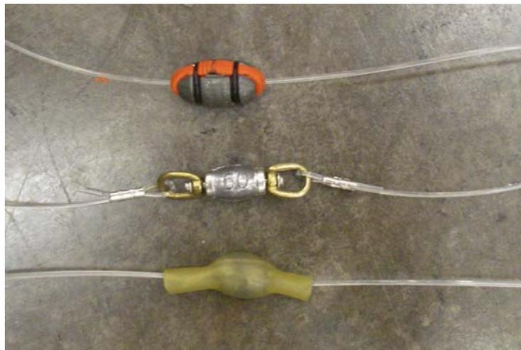
Fig. 1. Experimental FishTek-designed 'SafeLead' consisting of two pieces of lead, a rubber carrier in between the leads, and two O-rings (top), conventional lead center swivel (middle), and experimental egg lead inserter in rubber tubing (bottom).
