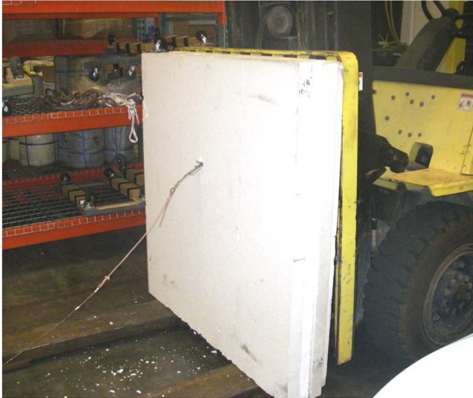
Fig. 4. Lead weights were projected at an EPS target at the “boat”-end of the branchlines.
