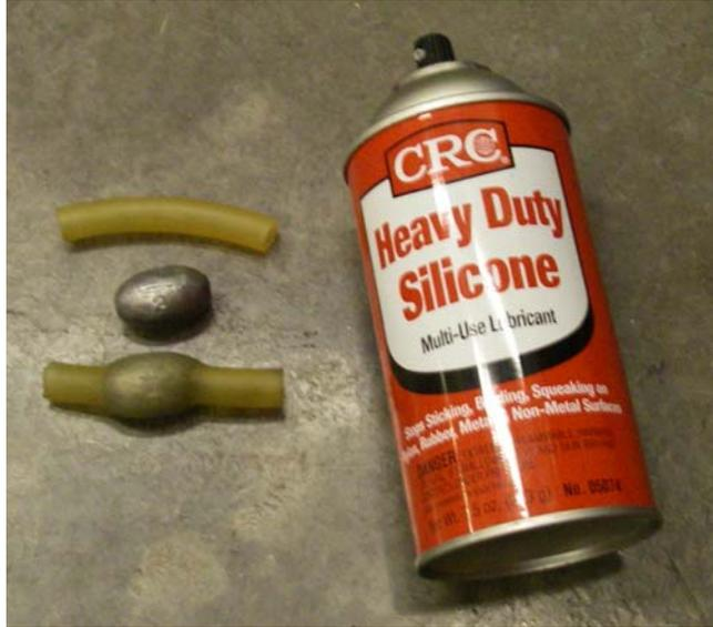
Fig. 2. One of the two experimental treatment leads, consisting of a 57 g egg lead inserted into thin-walled rubber tubing. Silicone was sprayed into the tubing before inserting the lead.
