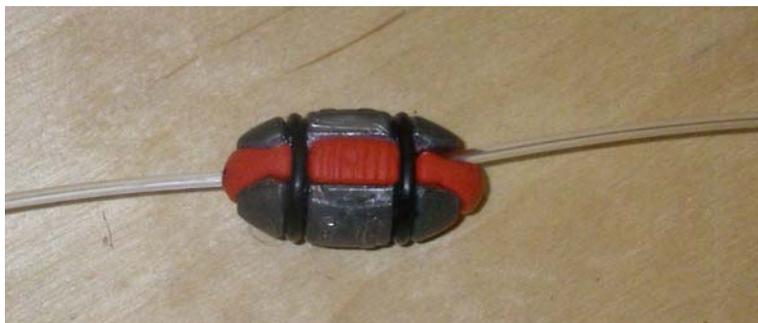
Fig. 6. Difficulty threading fishing line through the Safe Lead weight: line exits through the wall of the carrier rubber core.
