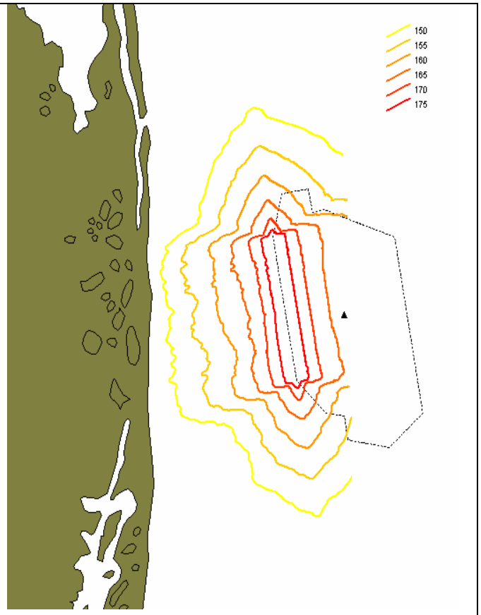
Figure 5.10 - Modelled envelope footprint of single-pulse SEL from all the individual shots along the most inshore survey line. Levels are in dB re \mu\text{Pa}^2\text{-sec} .
