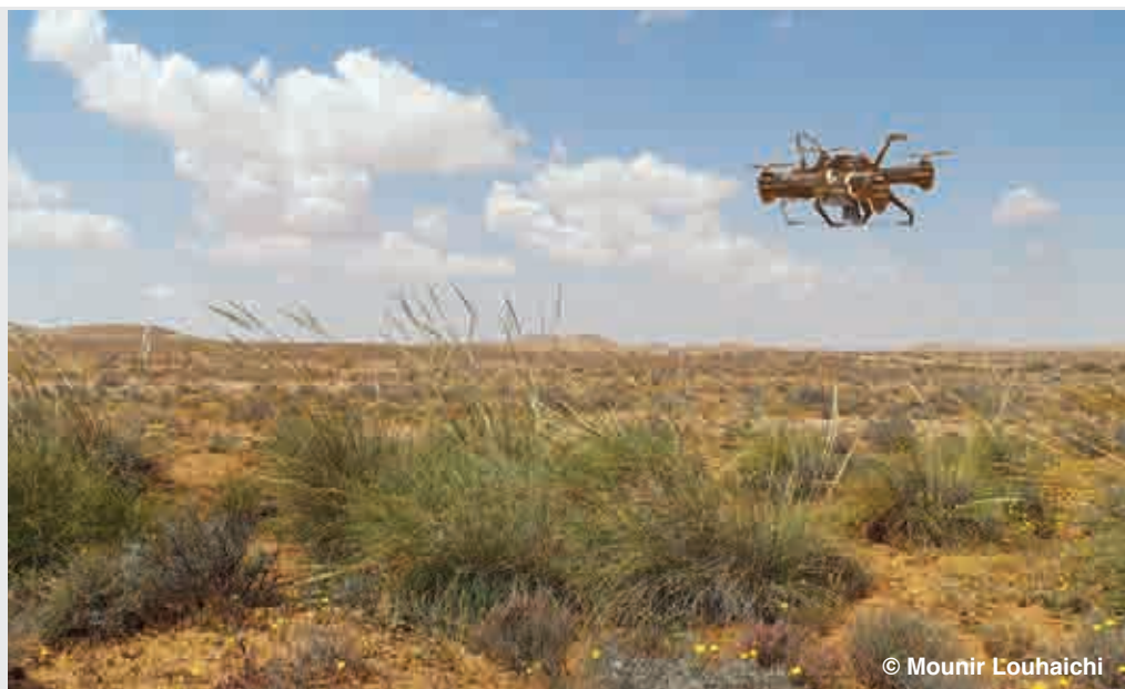
Figure 4. Precision aerial seeding for rangeland rehabilitation using drone
