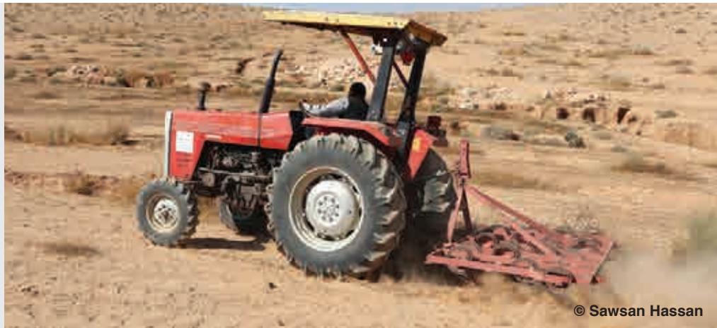
Figure 3. Using a crust breaking machine (cultivator) in the Jordanian Badia
