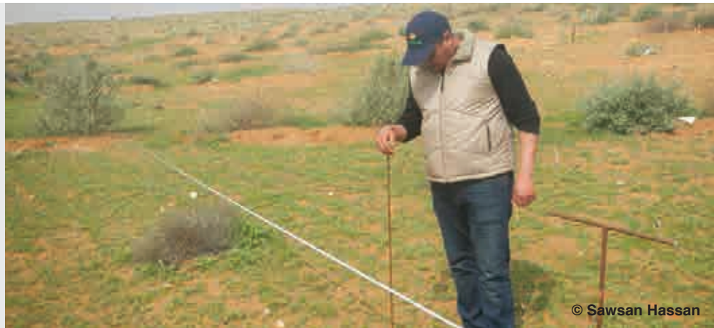
Figure 3. Vegetation cover estimation using the point intercept method
